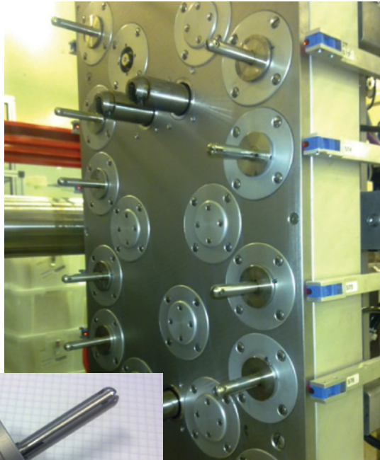
Figure 1: Mould modifications were required to successfully implement the unscrewing mechanism for this externally-threaded component
