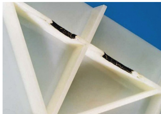
Figure 1: Burn marks caused on the ribs of this moulding are due to trapped gas
