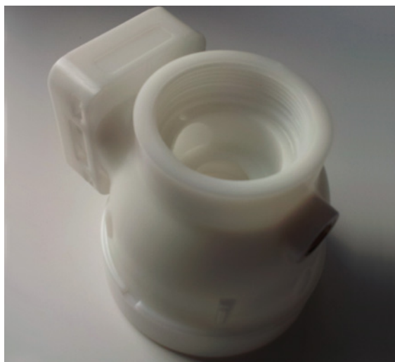
Figure 2: The thick wall sections in this POM water meter component design required a cycle time of around 120s. Switching to reinforced PA presented big cost reduction opportunities.
