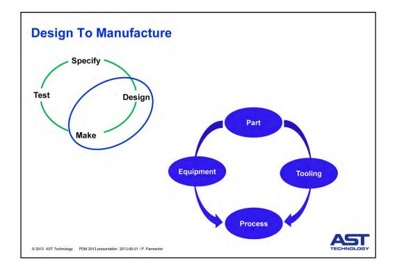
To Achieve an optimum manufacturing capability for an injection moulded component requires consideration of four key elements:
